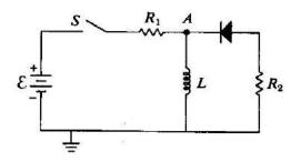
94. In the circuit shown above,  $R_2 = 3R_1$  and the battery of emf  $\mathcal{E}$  has negligible internal resistance. The resistance of the diode when it allows current to pass through it is also negligible. At time t = 0, the switch S is closed and the currents and voltages are allowed to reach their asymptotic values. Then at time  $t_1$ , the switch is opened. Which of the following curves most nearly represents the potential at point A as a function of time t?
